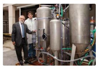
House in Colburn Laboratory, the biodiesel processor (worth an estimated \$50k) is capable of recycling 130-150 gallons of cooking oil per batch to produce 100 gallons of biodiesel fuel, as well as glycerin, a syrupy by-product with many uses in agriculture, pharmaceuticals and beauty products.
